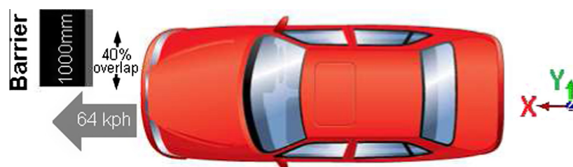
Fig. 1. A scheme for EuroNCAP Frontal offset crash tests [41].
